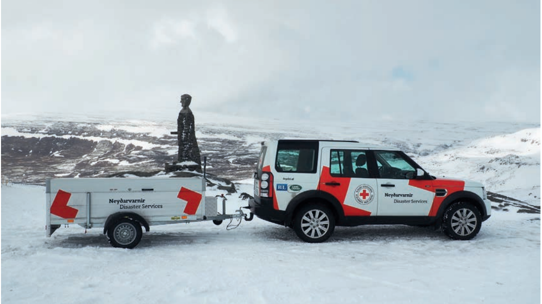
Figure 7 The Icelandic Red Cross has relief trailers with emergency shelter supplies in 20 locations around Iceland. The trailers are adjusted to be as low as possible to better withstand windy conditions in the Arctic. Photo: Finnish Red Cross/Sini Hangaslammi
