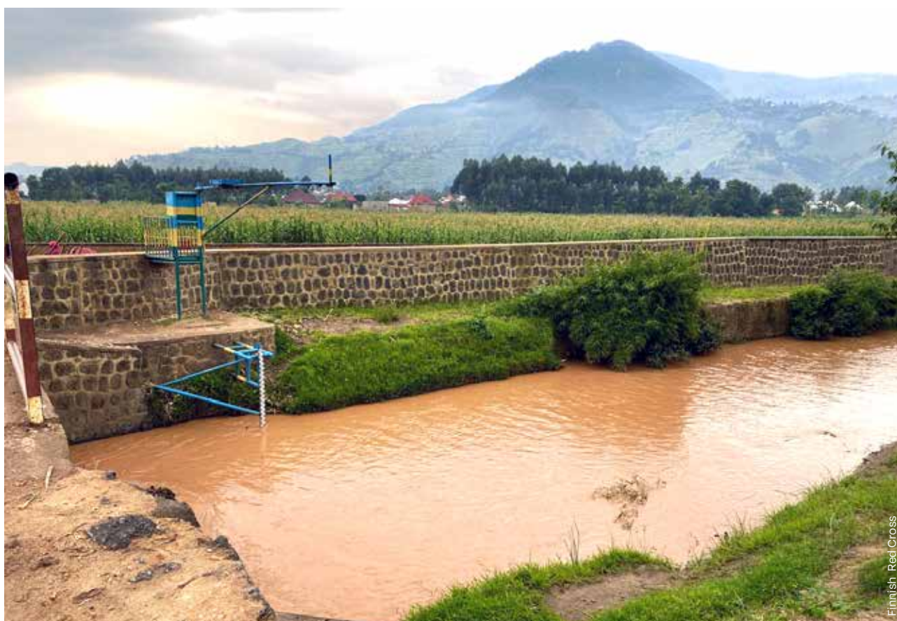
Telemetry station for water level measurement in Telimbere, Nyundo sector, Rwanda.
